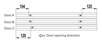
Fix the bracket fixing piece on the corresponding door according to the figure, and pay attention to the direction of the door and the distance between both sides;
