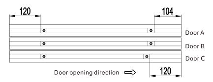
Fix the bracket fixing piece on the corresponding door according to the figure, and pay attention to the direction of the door and the distance between both sides;
